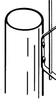
On wood masts, use long brass wood screws.
